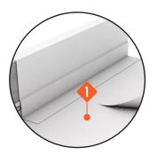
Waterproofing membrane: FLAGON EP/PR ENERGY PLUS
