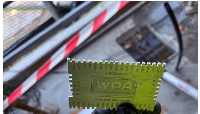
Pic 5. A Wet Film Thickness gauge helps to create even application
