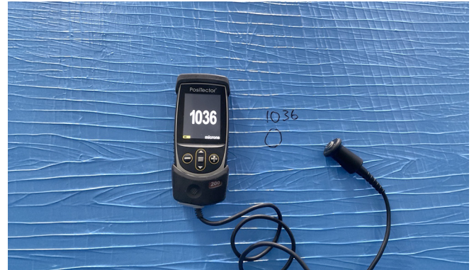
Pic 4. Use tools like a PosiTector to achieve the required thickness
